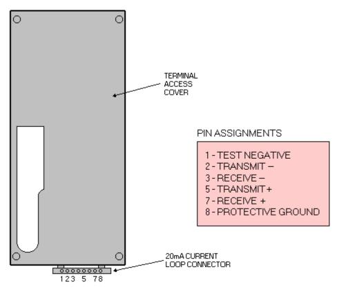
Figure 2-3 20 mA Current Loop Interface
