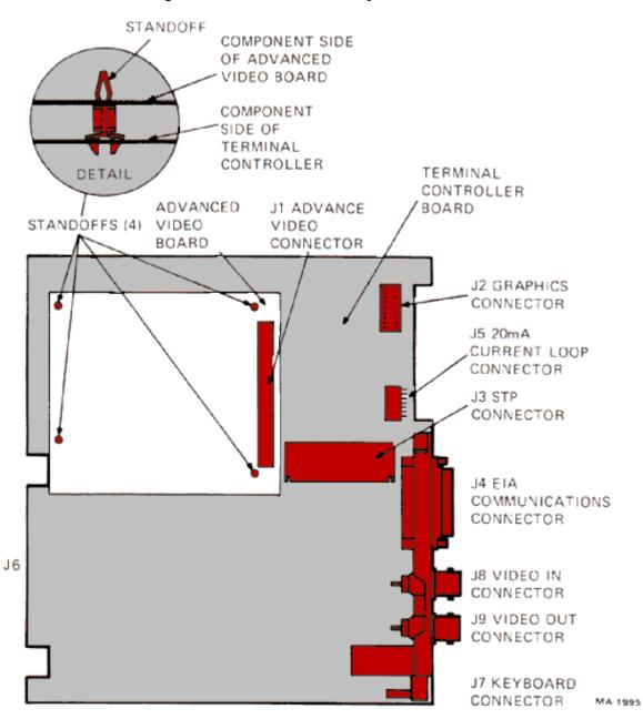
Figure 4-2 Advanced Video Option Installation
